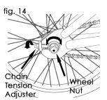
b. If the wheel is equipped with chain tension adjusters (fig. 14) loosen the nuts on the adjusters by turning both counterclockwise with a correctly sized open end or adjustable wrench an equal number of turns. This allows you to move the wheel as required by step (4) below.
