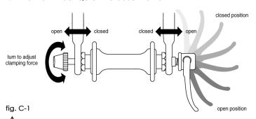
WARNING: Riding with an improperly adjusted wheel quick release can allow the wheel to wobble or disengage from the bicycle, causing serious injury or death to the rider. Therefore, it is essential that you:
